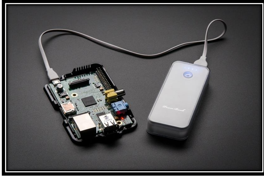
Figure 2: Connection between the Raspberry Pi and the Battery with Red LED and Blue Lights On Take the micro-USB connector out of the Raspberry Pi. Now we want to make the connection between the 4D Display and the Raspberry Pi.
